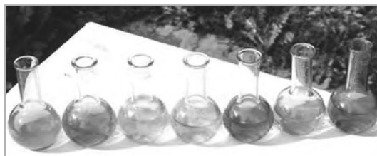
Fig. 8.5: Colours of some of the first row transition metal ions in aqueous solutions. From left to right: V^{2+} , V^{3+} , Mn^{2+} , Fe^{3+} , Co^{2+} , Ni^{2+} and Cu^{2+} .
